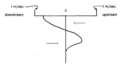
The flow downstream in the upper layer in the middle of the estuary is usually much greater than the river flow alone, because the salt water mixed from depth must flow out at the surface as well.
