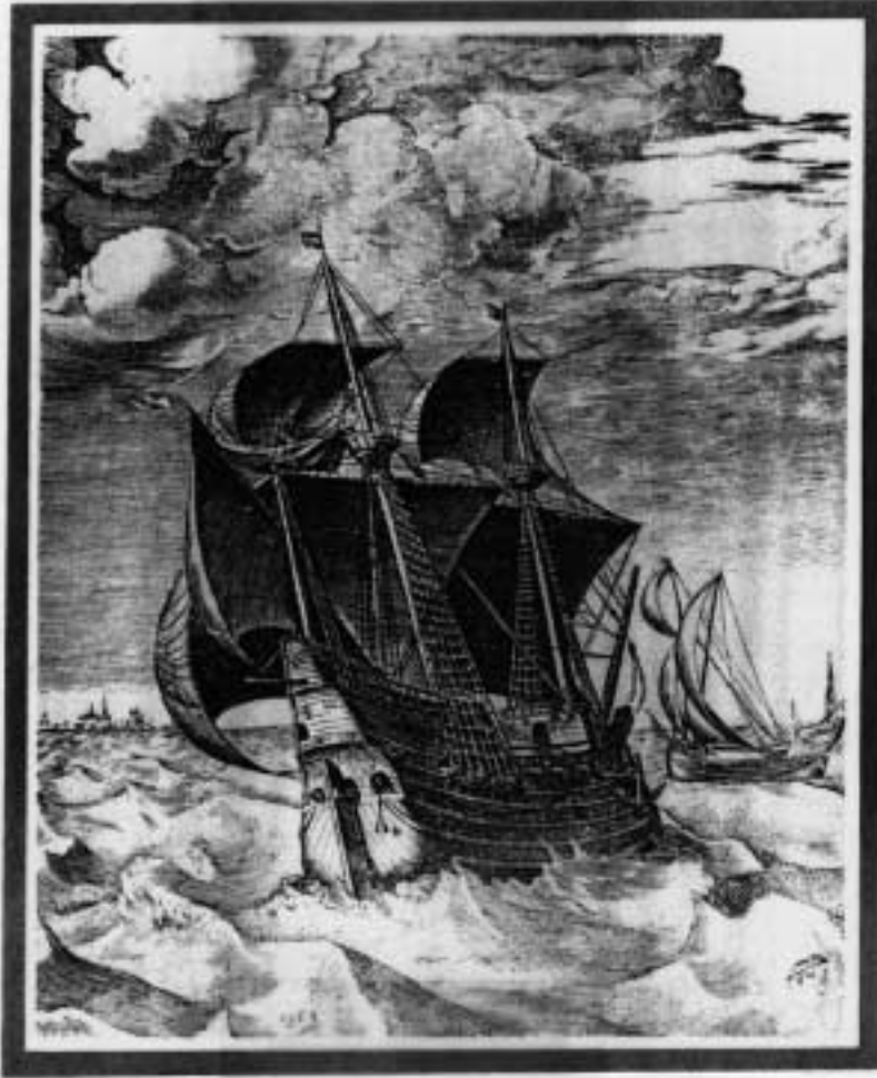
Figure 7-1. “A Flemish version of the machine with which the {European mariners} changed the world: the three-masted ship, square-rigged on the foremast and main-mast, lateen-rigged on the mizzmast, with smaller vessel in sight” (Crosby, 1986: Plate 2).
